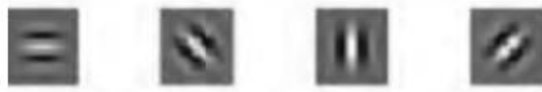
Figure 4. Gabor filter with different orientations ( 0^\circ , 45^\circ , 90^\circ , 135^\circ ) for MRI images.
